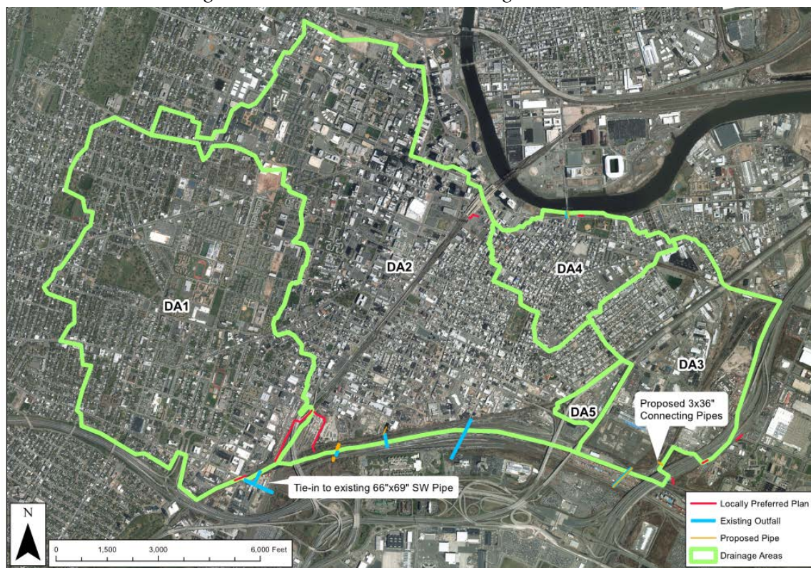
Figure 24: Passaic Tidal Project Existing and Recommended Interior Drainage Features
